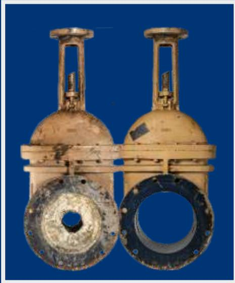
Without effective water treatment, a cooling water system can suffer from scale formation, corrosion and fouling and may become a breeding ground for harmful bacteria such as those which cause Legionnaires' Disease. This reduces efficiency, shortens plant life and makes your operation unreliable and unsafe
